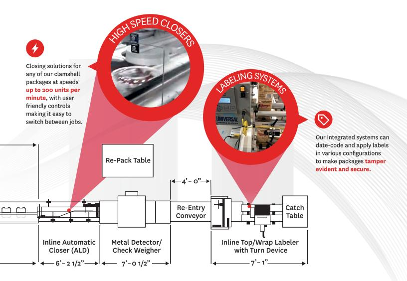
We can develop an entire packaging line or design around existing equipment.
