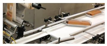
We can automate vibrating the containers to settle food; we can flip the container around onto its lid, or turn containers to the desired position for labeling or ink-jetting.
