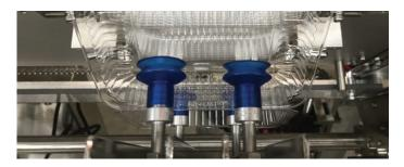
Inline equipment is designed to pick and place empty containers onto a packing conveyor quickly, accurately, and efficiently.
