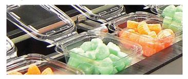
Container closing equipment is available for all Inline clamshell containers; closing at rates up to 200 units per minute or more. Change over from one size container to the next takes only minutes.
